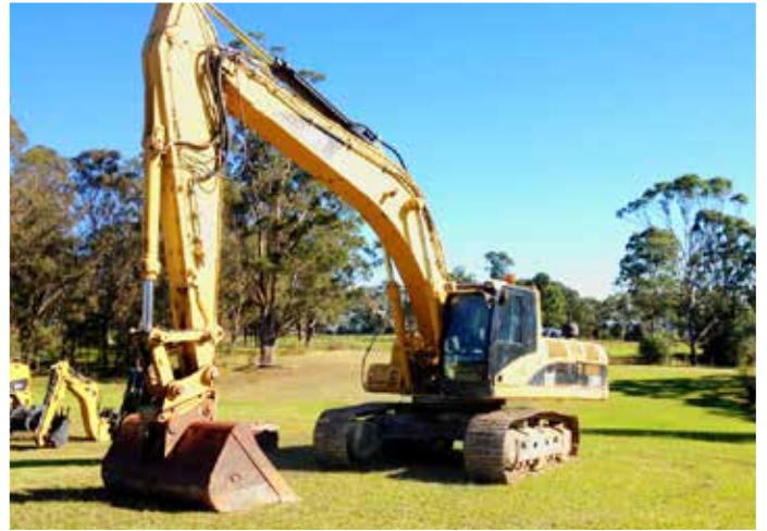
CAT 330C EXCAVATOR
